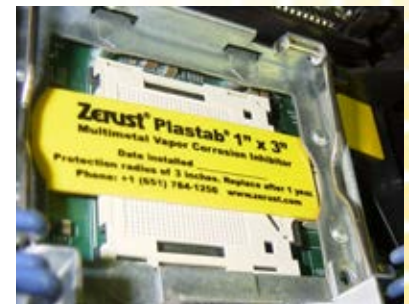
Plastabs fit and protect small spaces.
